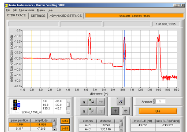
A typical trace with the v-OTDR
